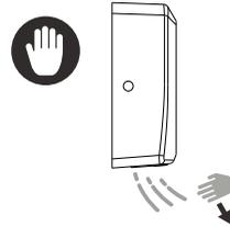
After 3 seconds without detecting hands, the device stops automatically.
