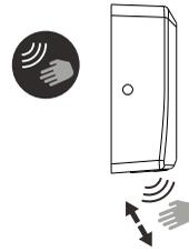
It is possible to adjust the sensor range by means of the sensor VR located on program PCB (See section 8 in "INSTALLATION").
